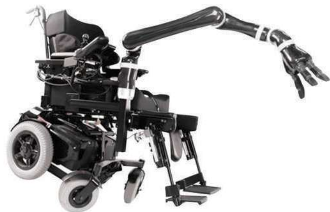
Figure 3: JACO robotic arm mounted on an electric wheelchair [49]
