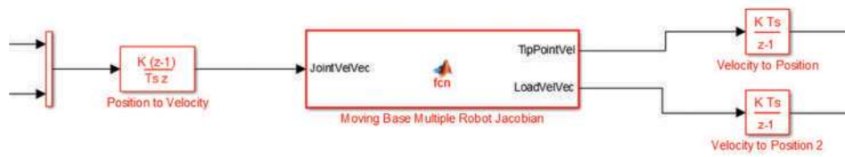
Figure 4: Simulink block diagram of the robot Jacobian
